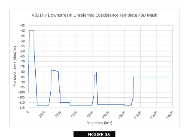
V811Hv Downstream Unreferred Coexistence Template PSD Mask
