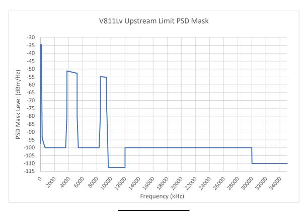
FIGURE 22 V811Lv Upstream Limit PSD Mask
