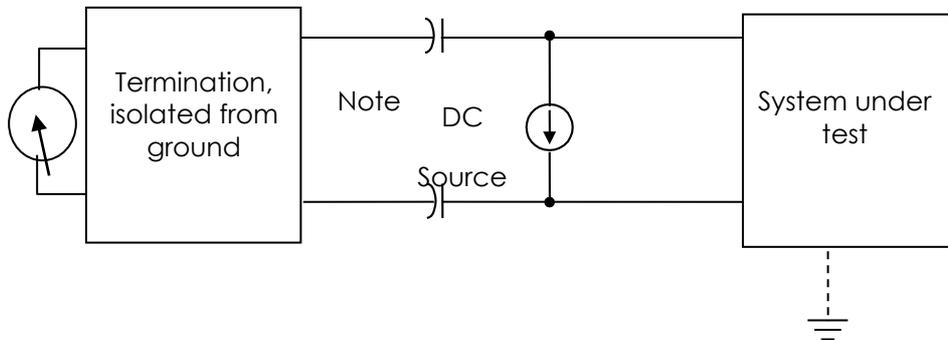
*NOTE: The measurement uncertainty needs to take into account the accuracy of the differential termination, including the effect of the blocking capacitors and other equipment.*
