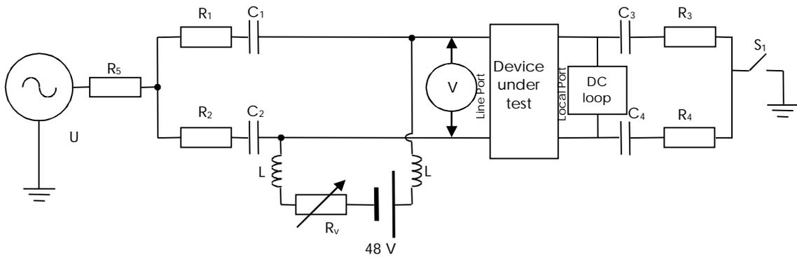
Figure 3(a) Test for xDSL filter balance about earth at the Line Port
