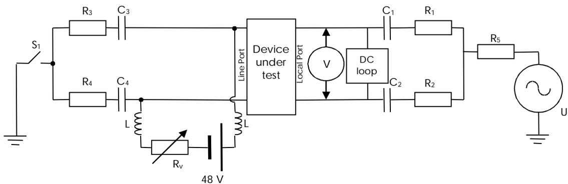
Figure 3(c) Test for xDSL filter balance about earth at the Local Port
