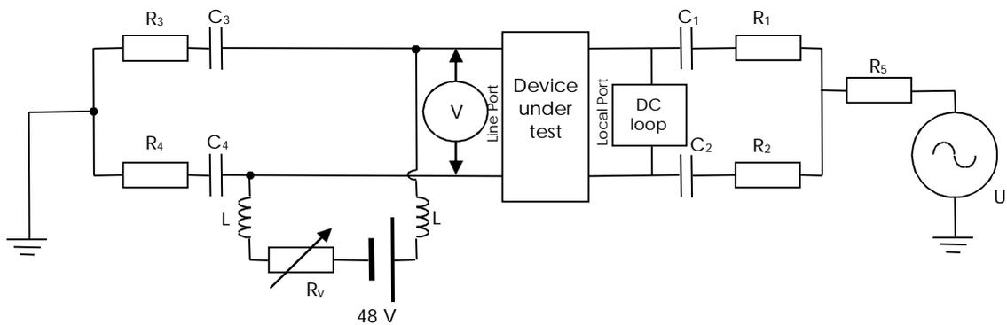
Figure 3(b) Test for xDSL filter balance about earth from the Local Port to the Line Port
