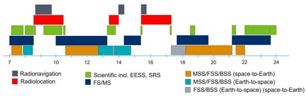
Figure 1: Frequency allocations with the 7-24 GHz range
