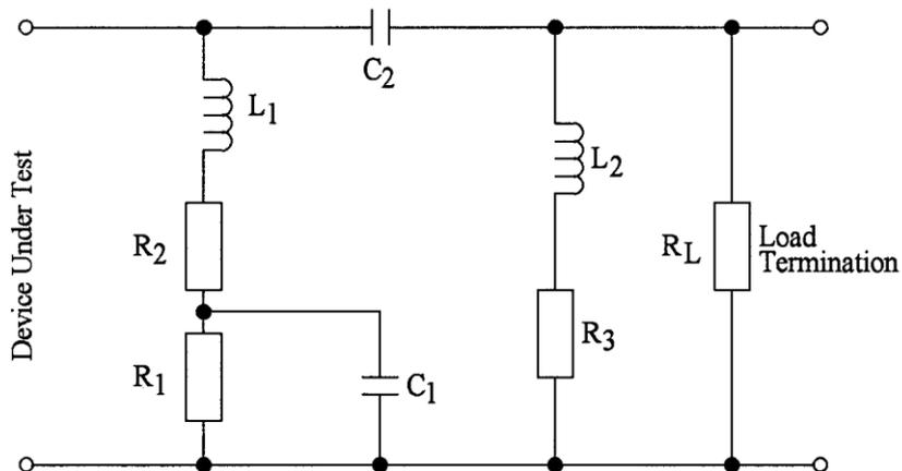
$L_1 = 4 \text{ H} \pm 20\%$  up to 125 mA d.c. over the range 100 Hz to 4000 Hz
