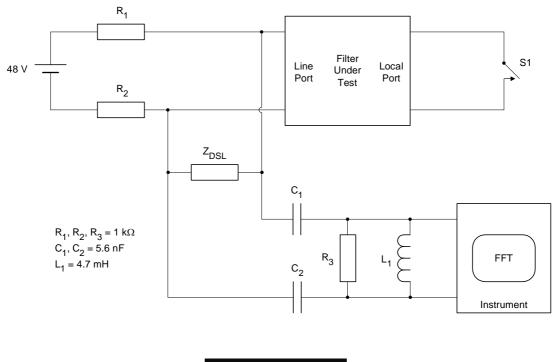
Figure 6 Test for PSTN transient effects
