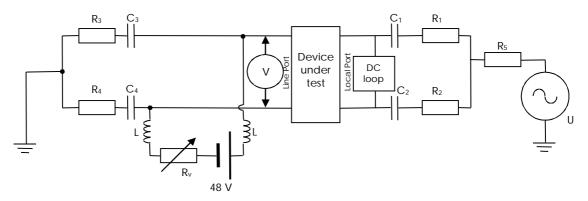
Figure 3(b) Test for xDSL filter balance about earth from the Local Port to the Line Port
