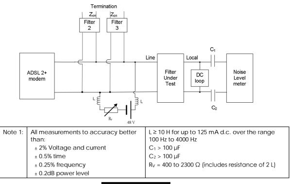
Figure 5 Psophometric noise measurements
