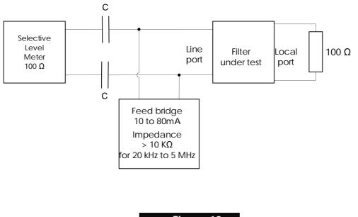
Figure 12 xDSL band noise measurements
